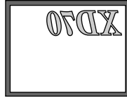
“Vertical Flip” Off “Horizontal Flip” On
